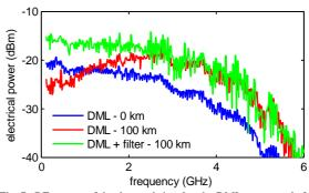
Fig. 7. RF spectra of the detected signal at the DML output and after transmission over 100 km SSMF without and with filter.
