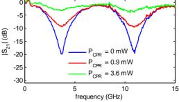
Fig. 3. Filter frequency responses when the PhC coupler is tuned.
