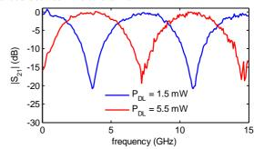
Fig. 4. Filter frequency responses when the PhC delay line is tuned.
