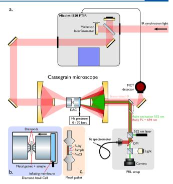
**Figure 3.** (a) Scheme of the optical setup used to obtain infrared spectra of the HgX nanocrystals under pressure. Synchrotron light is used as broad band infrared source. The pressure within the diamond cell is measured through the shift of the ruby luminescence. DAC: diamond anvil cell. PRL: pressure by ruby luminescence spectrometer. DM: dichroic mirror. (b) Scheme of DAC. (c) Scheme of the inner part of the DAC containing the actual nanocrystal sample.
