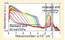
blende phase up to 3 GPa. Under compressive strain, the interband signal blue-shifts by 60 meV/GPa, while the intraband transition red-shifts by a small amount (8 meV/GPa). Using an 8-band k·p formalism, we reveal that the interband shift has the same origin as the one observed for bulk material (change of effective mass, followed by band gap opening), while the intraband shift can be attributed to an increase of effective mass only.
