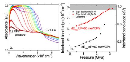
Figure 4. (a) Infrared spectrum of HgTe CQDs, with a zero-pressure band edge around  $6000 \text{ cm}^{-1}$ , under increasing pressure. (b) Interband bandedge energy as a function of the applied pressure for two populations of HgTe CQDs: with a band edge around  $4000 \text{ cm}^{-1}$  (HgTe 4k, in black) and with a band edge around  $6000 \text{ cm}^{-1}$  (HgTe 6k, in red). In the 1-2 GPa range, where a linear fit is possible (dashed lines), the value of dE/dP is indicated.
