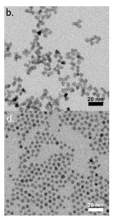
Figure 1. (a) Infrared spectra of two different sizes (6 and 8 nm) of HgTe CQDs, under zero pressure. (b) TEM image of HgTe CQDs with a band-edge energy at 4000 cm<sup>-1</sup>. (c) Infrared spectra of three different sizes (5, 6, and 15 nm) of HgSe CQDs, under zero pressure. (d) TEM image of HgSe CQDs with an average size of 5 nm presenting an intraband transition at 2500 cm<sup>-1</sup>.
