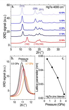
Figure 2. (a) Diffraction pattern of HgTe CQDs (with a band edge at zero pressure at 4000 cm<sup>-1</sup>) under different pressures. (b) Zoom on the (111) Bragg reflection of HgTe CQDs (with a band edge at zero pressure at 4000 cm<sup>-1</sup>) under different pressures while the material remains in the zinc blende phase (i.e., P < 4 GPa). (c) Lattice parameter of the zinc blende phase as a function of pressure.
