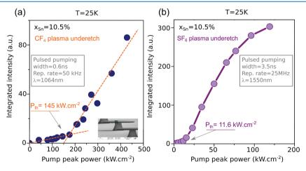
**Figure 4.** (a) L–L curve obtained at 25 K from a 10  $\mu$ m diameter microdisk with 10.5% of Sn underetched with a CF<sub>4</sub> plasma. The dashed lines are drawn to guide the eyes. The inset shows a SEM image of such microdisks. (b) L–L curve obtained at 25 K from a 8  $\mu$ m diameter microdisk fabricated from the same epitaxial layer with 10.5% of Sn but underetched with a SF<sub>6</sub> plasma.
