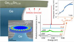
reproducible lasing thresholds around 10 kW cm<sup>-2</sup>, lower by 1 order of magnitude as compared to the literature. These results were obtained after the removal of the dense array of misfit dislocations in the active region of the GeSn microdisk cavities. The results offer new perspectives for future designs of GeSn-based laser sources.
