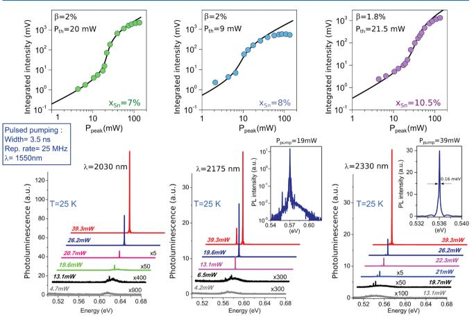
Figure 3. (Bottom) Pulsed peak power dependence of emission spectra for 4  $\mu$ m diameter microdisks with Sn contents between 7% to 10.5% with corresponding L–L curves at 25 K. (Top) The continuous curves in the figures on top are calculated curves using the laser rate equations with the indicated thresholds and  $\beta$  factors. The insets show typical spectra above the lasing threshold.
