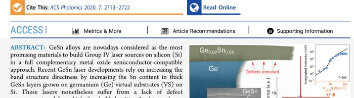
management and from high threshold densities. In this work, we examine the lasing characteristics of GeSn alloys with Sn contents ranging from 7% to 10.5%. The GeSn layers were patterned into suspended microdisk cavities with different diameters in the 4-8  $\mu$ m range. We evidence a direct band gap in GeSn with 7% of Sn and lasing at 2–2.3  $\mu$ m wavelength under optical injection with
