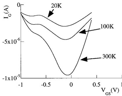
FIG. 5. Gate current vs gate voltage at temperatures 20, 100 and 300 K for  $V_{DS}=3$  V.
