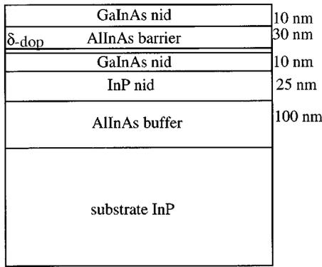
FIG. 1. Layer structure of the composite channel HEMT.
