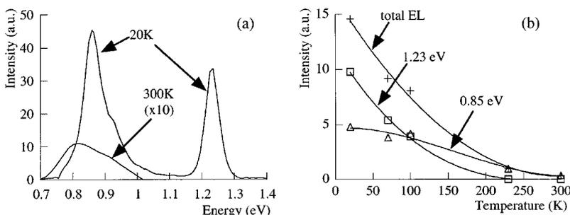
FIG. 3. (a) EL spectrum at 20 and 300 K for  $V_{DS} = 3$  V and  $V_{GS} = 0$  V. (b) EL intensity vs temperature for  $V_{DS} = 3$  V and  $V_{GS} = 0$  V.
