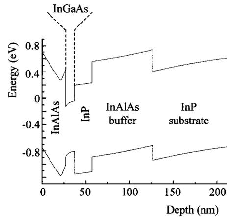
FIG. 2. Conduction and valence bands of the composite channel HEMT calculated by numerical simulation of Poisson equation.
