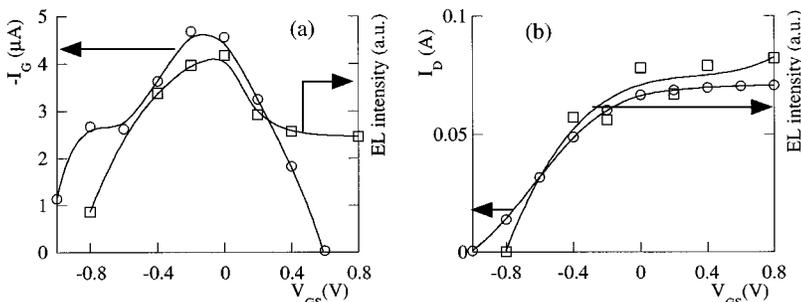
FIG. 6. (a) Gate current (circle) and EL intensity of the 0.85 eV line vs (square) gate voltage for  $V_{DS}=3$  V at temperature 100 K. (b) Drain current (circle) and EL intensity of the 1.25 eV line (square) vs gate voltage for  $V_{DS}=3$  V at temperature 100 K.
