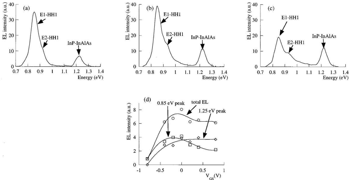
FIG. 4. EL spectra at 100 K for  $V_{DS}=3$  V and  $V_{GS}=-0.4$  V (a),  $V_{GS}=0$  V (b),  $V_{GS}=+0.4$  V (c). Integrated EL intensity of each line and of the total EL spectrum vs  $V_{GS}$  for  $V_{DS}=3$  V (d).
